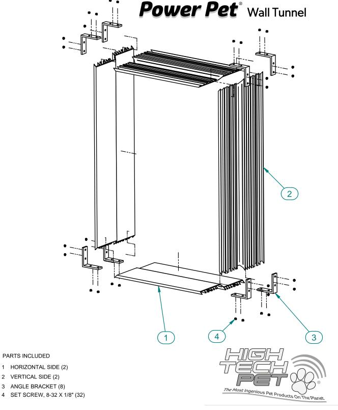
Insert angle brackets at each corner. Line up sides and tighten the set screws.
