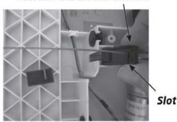
16) Insert the sandwiched cable guides into the guide slot of the frame just below the motor pulley.
