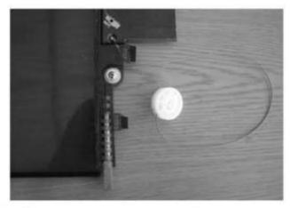
Remove screw and small pulley on panel
