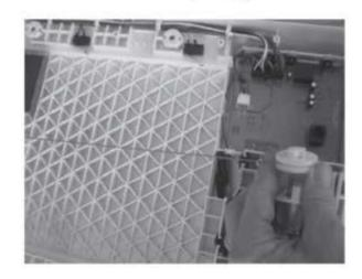
13) Place the pulley over the motor shaft, align the shaft slot with the pulley slot (by rotating the motor shaft with a pair of pliers if necessary) and press the pulley on the shaft as shown. Leave a small gap between the pulley and the plastic motor bracket, as shown.
