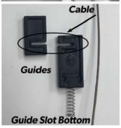
17) Finally, remove any slack in the cable by winding the pulley (turn with your fingers or pliers). Re-attach the rear frame using six flat head screws at the top of the door, and pan head screws around the rest of the door frame. Do not over tighten the screws.
