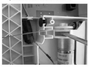
5) Pull metal latch and spring completely off the door panel.
