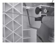
15) Sandwich the small cable guide next to the large cable guide with the slot in the OPPOSITE direction as the large cable guide slot. This captures the cable from both sides.
