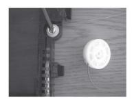
13) Gently stretch the cable up to the motor. Wind up any extra cable on the pulley.
